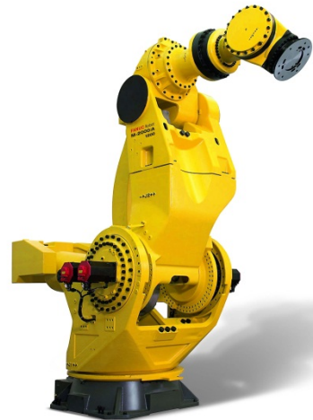
1,200 kg payload capacity - Handling of largest parts and structures
